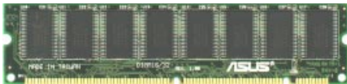
Non-ECC SDRAM DIMM (8 chips) 64bits
